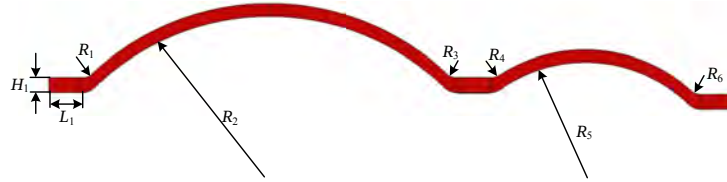
Figure 26: Geometric configuration and dimensional parameters of Al bonding wire.
